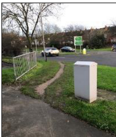
Photo (Southbound): trodden path to carriageway edge on north side; crossing on Thorndike Way Arm
